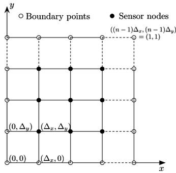
(a) An  $n \times n$  grid network for the solution of Poisson's equation
