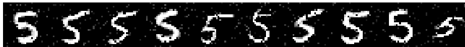
Figure 2: A set of ten “5”-digit images corrupted by a salt-and-pepper noise of density 0.1 (first row), on which we applied the kernel PCA for data denoising. The pre-image results using the fixed-point iterative algorithm [10] are illustrated (second row), the MDS technique [11] (third row), the non-negative gradient pre-image (6) (fourth row) and the non-negative pre-image with the iterative schema (7) (last row).
