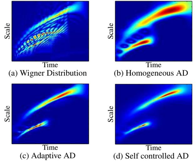
**Fig. 2.** The two conductance functions succeed in providing a sharp, concentrated and clean representation for this signal composed of two power laws.
